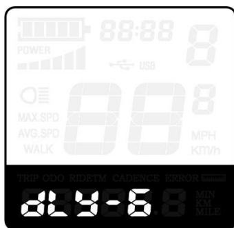
Delay Time of Battery Power Interface
